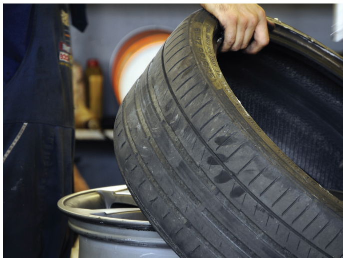
Example of a non-roadworthy tyre. Tread limit below 1 mm.
